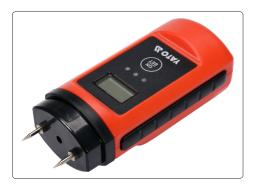
0.2-2.9% WALL/MASONRY 6-60% WOOD 10 mm MAX SENSE DEPTH
